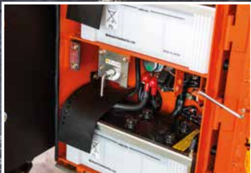
Easy access battery compartment
