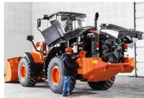
Easy access to the engine compartment.
