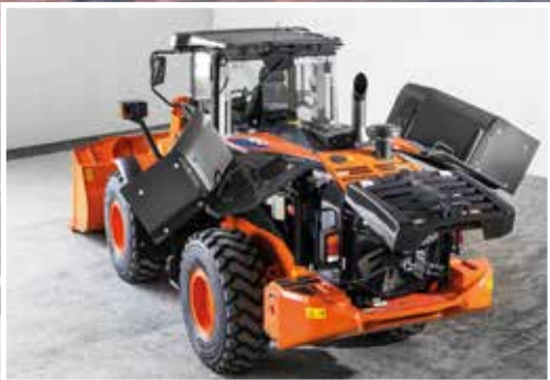
Ground level access for easy maintenance.
